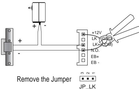
set to Normally Closed on the Unlock Relay mode on DT-config software.
