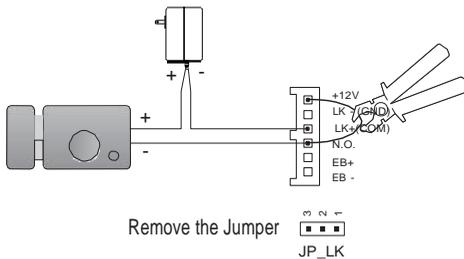
set to Normally Open on the Unlock Relay mode on DT-config software.(default)
