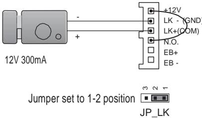
set to Normally open on the Unlock Relay mode on DT-config software.
