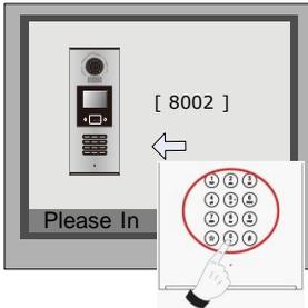
Press “#”, Input “8002”, then input Setup Code or Admin Code
